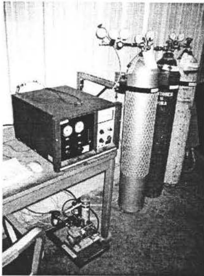
Figure 3.23 NO/NO x Analyzer System.
