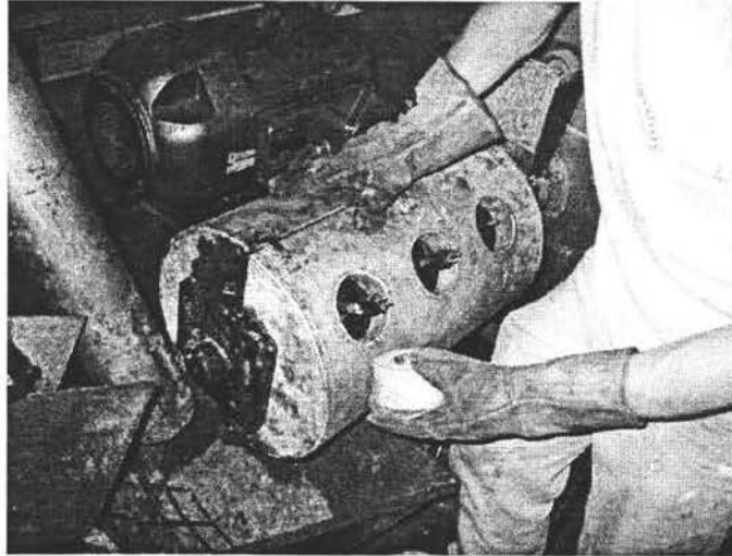
Figure 6. Securing Extruder Barrel Heat Shield
